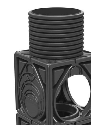
Once the main access chamber has been constructed it will be necessary to add a 18" (450mm) ID raising piece cut to length and placed over the top of the access chamber unit. Once the bases of the upper module(s) have been removed, simply stack units on top of each other ensuring that each module is clipped to the main structure using the StormBrixx® layer connectors.
