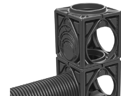
Once the main access chamber has been constructed it will be necessary to add a 18" (450mm) ID raising piece cut to length and placed over the top of the access chamber unit. Once the bases of the upper module(s) have been removed, simply stack units on top of each other ensuring that each module is clipped to the main structure using the StormBrixx® layer connectors.
