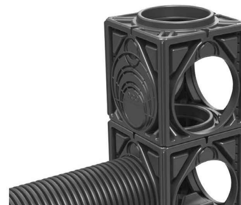
Once the main access chamber has been constructed it will be necessary to add a 18" (450mm) ID raising piece cut to length and placed over the top of the access chamber unit. Once the bases of the upper module(s) have been removed, simply stack units on top of each other ensuring that each module is clipped to the main structure using the StormBrixx® layer connectors.
