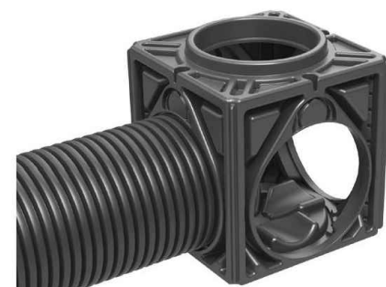
Cut unit at guides for required pipe connection. Push up to 2.5' (65mm) of pipe into access chamber module.
