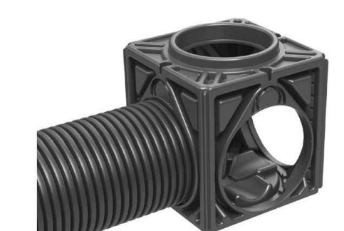
Cut unit as guides for required pipe connection. Push up to 2.5" (65mm) of pipe into access chamber module.
