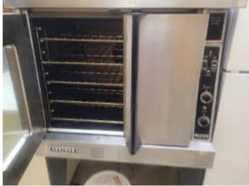
Convection Oven. Excellent for baked goods. Air circulates heat while cooking. On the side panel are the temperature and timer knobs as well as switches for off/on and heat/cooling off settings. Temperature light turn off when the oven is up to temperature. Rack slide in and out for easy removal of hot pans.
