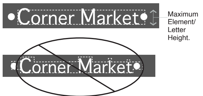
Figure 5-2: Measuring Wall Signs
