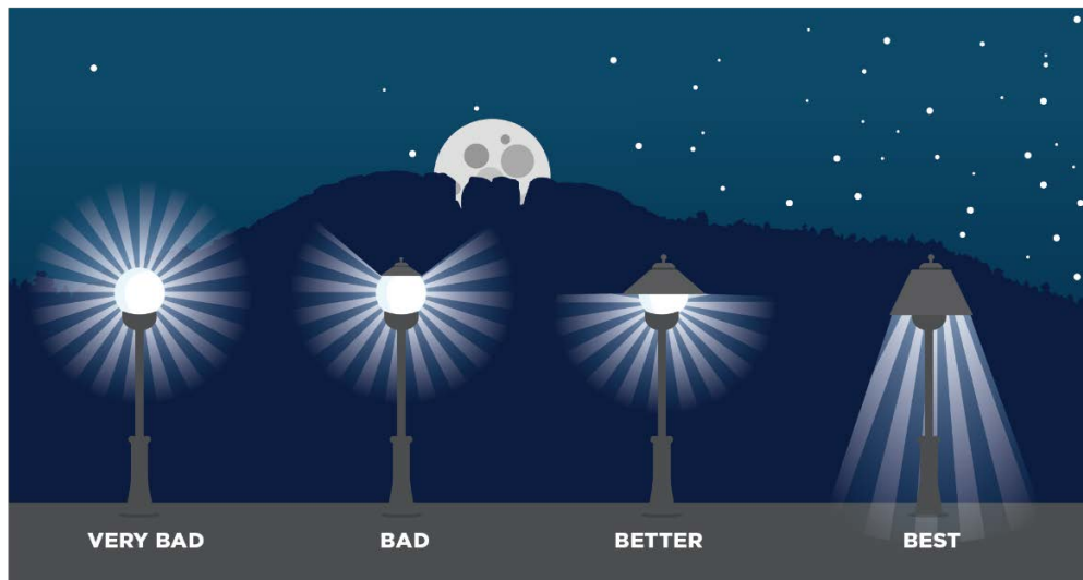
Figure 1A: Examples of Appropriate (“best”) and Inappropriate Light Shielding
