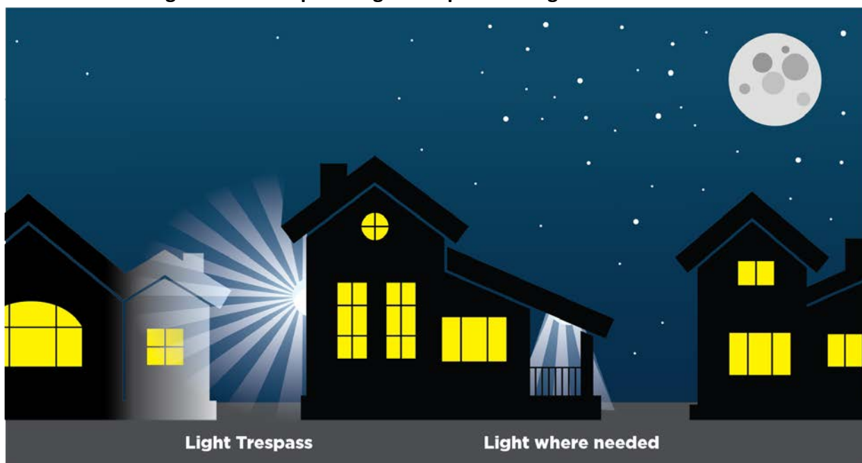
Figure 1E: Example of Light Trespass and Light Where Needed
