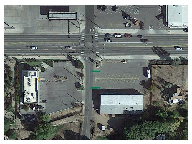
CR104 is currently stop-controlled. Delay analysis indicates that additional capacity is limited for 2<sup>nd</sup> order movements (right turn out, left turn in), and severely limited for the 3<sup>rd</sup> order movement (left turn out). This will push trip distribution from SAN mainly to CR107.
