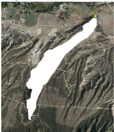
Drainage basin 3 outfalls to the alluvial fan on the east end of city property. Following the same methodology as Basin 2, the 100-year design flow is 68 cfs. An appropriately sized culvert and rip rap channel should convey this basin to the wetlands adjacent to the South Arkansas River.
