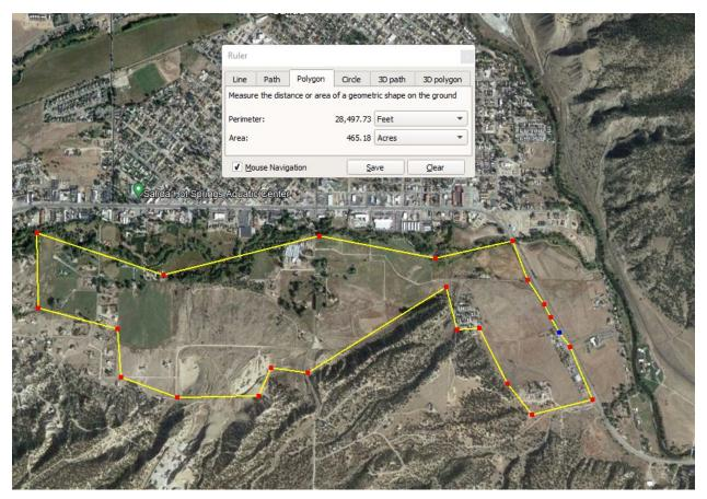
Removing parcels downstream (east) of SAN, by the same assumptions, 12" sanitary sewer interceptor is adequate for 350 acres of development. The interceptor should be 12" to the Wikoff (or Armstrong) property line to allow for 2.7 cfs peak flow with a minimum grade of 0.6%.
