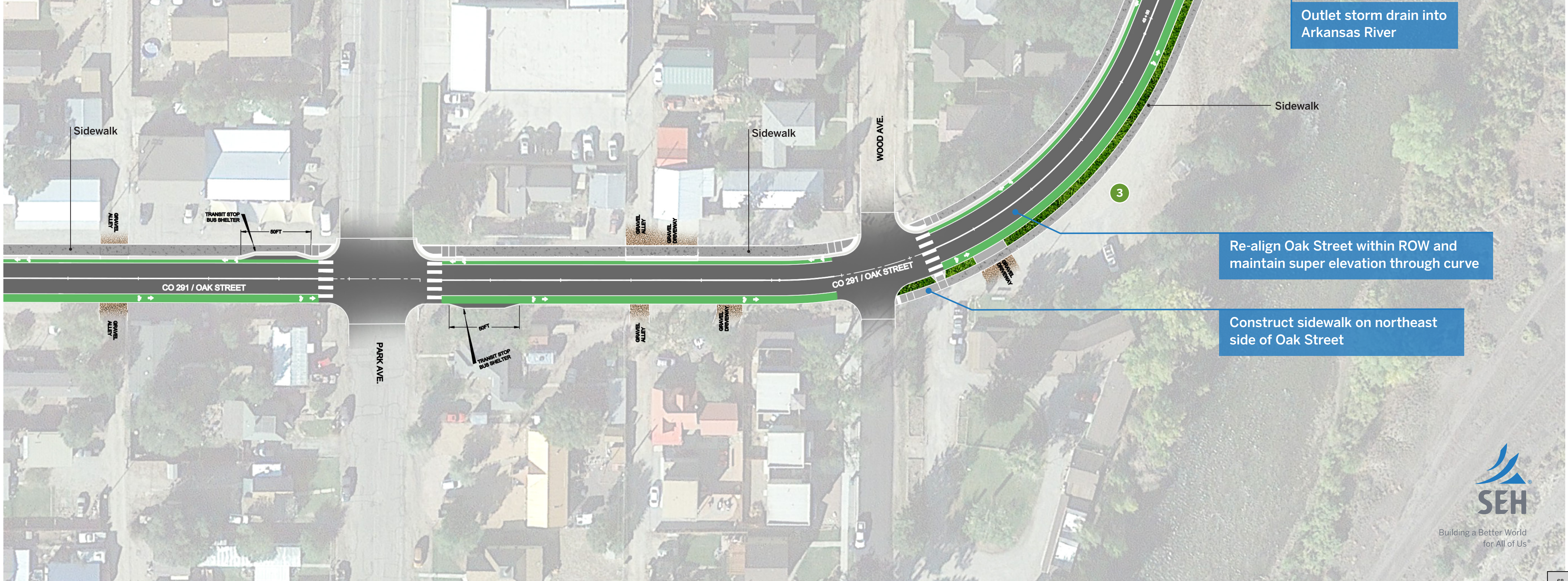
3 CO 291 will be realigned more centered in the ROW footprint. The curve pictured will be realigned to the right (East), with a new detached sidewalk.
