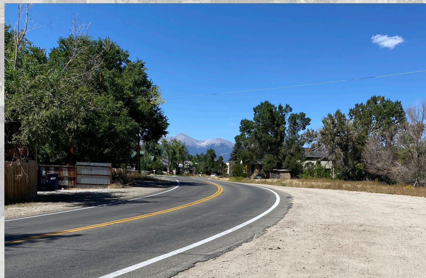
3 CO 291 will be realigned more centered in the ROW footprint. The curve pictured will be realigned to the right (East), with a new detached sidewalk.
