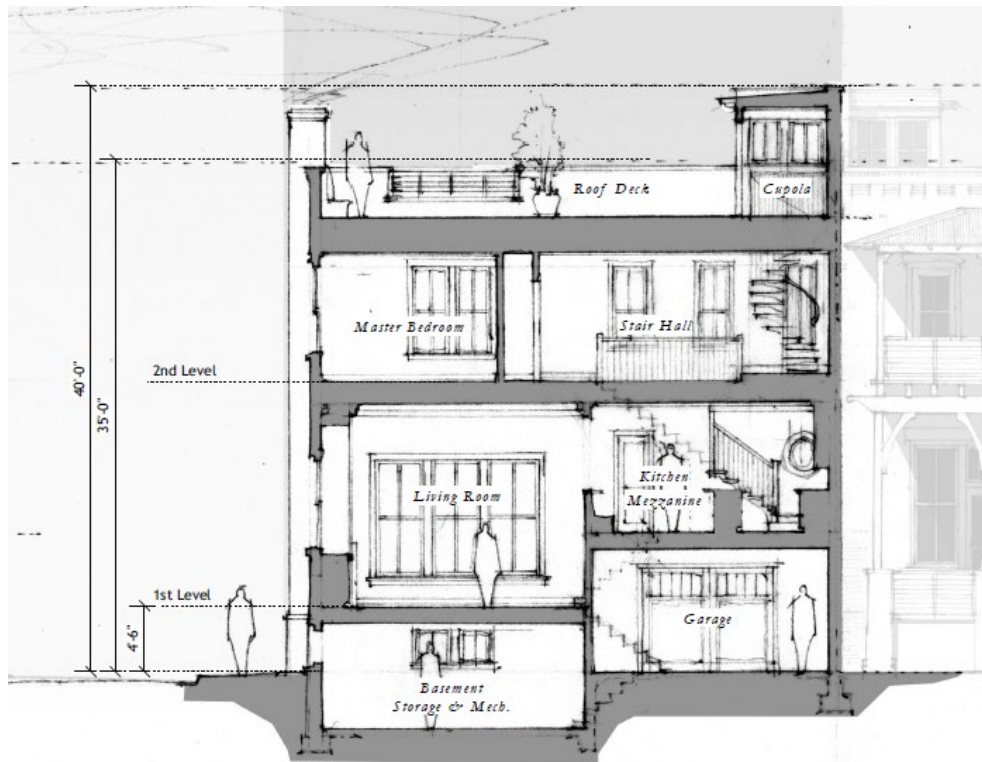
Concept of Unit 6 illustrating a portion at 2.5 story and a portion at 3 story
