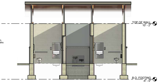
5 Section 6 - EW THROUGH RESTROOMS 1/4" = 1'-0"
