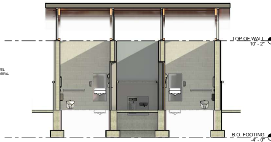
5 Section 6 - EW THROUGH RESTROOMS 1/4" = 1'-0"
