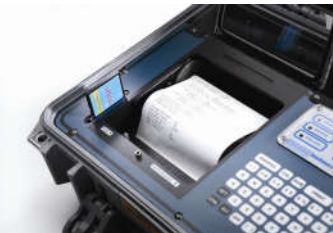
Removable 128 MB CompactFlash™ memory card able to record 10,000 full waveform events.
