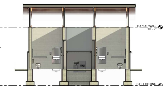
5 Section 6 - EW THROUGH RESTROOMS 1/4" = 1'-0"
