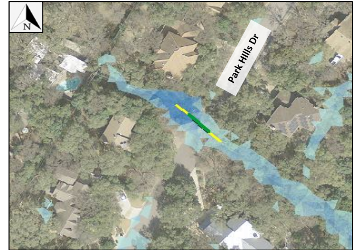
Proposed culvert in green. Channel improvements in yellow. Existing 100-yr inundation shown.
