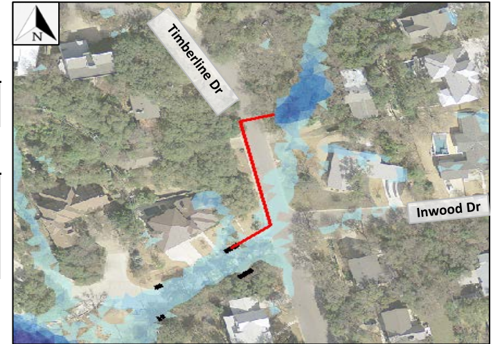
Proposed storm sewer in red to existing inlets in black. Existing 100-yr inundation shown.
