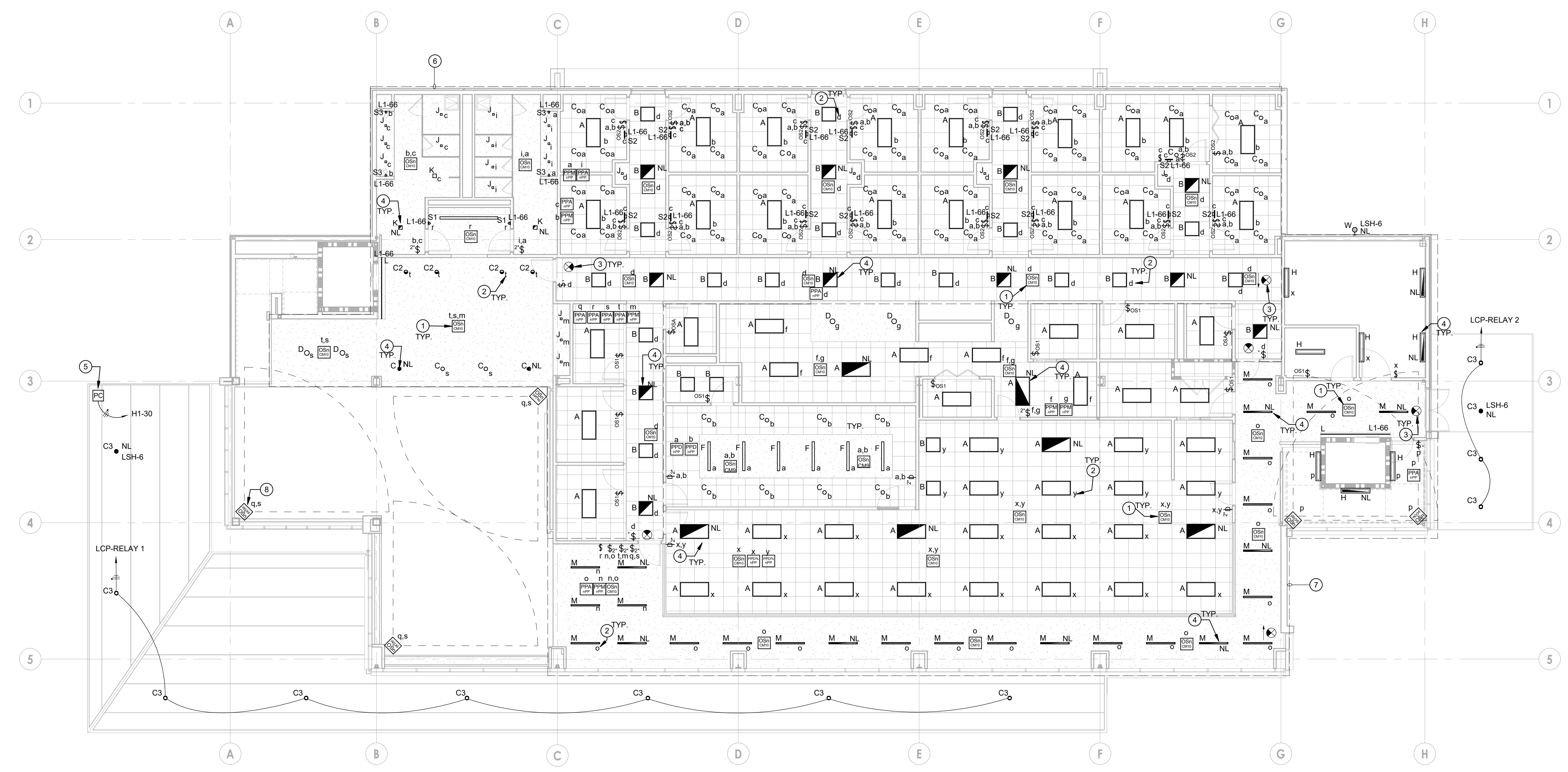
1 LEVEL 1 REFLECTED CEILING PLAN - LIGHTING 1/8" = 1'-0"
