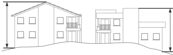
Figure 2-7: Maximum Overall Building Height
