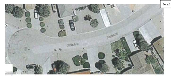
**Repair:** Chip-seal **Area:** 11,237 SF (W27' X L230' X 40'R)
