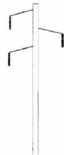
Figure 1 Typical Vertical Monopole Structure
