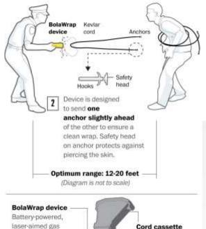
Cord cassette Lightweight 7 1/2-foot Kevlar cord can wrap around a typical body one to three times.
