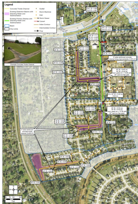
Proposed drainage improvement plan for area on city's west side.
