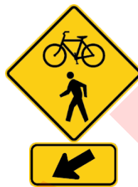
Figure 4-3, Current MUTCD-Standard Trail Crossing Assembly
