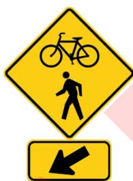
Figure 4-3, Current MUTCD-Standard Trail Crossing Assembly
