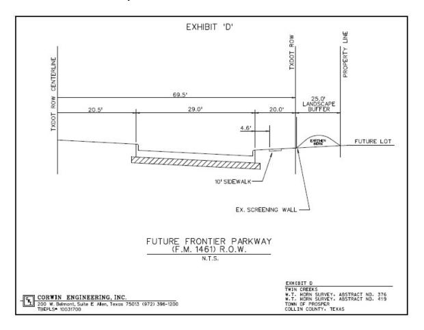
Above is the cross section from the TXDOT plans for the section of the expanded roadway in front of Twin Creeks.
