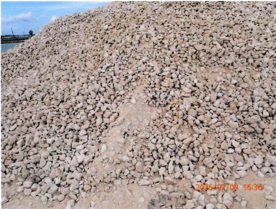
Figure 3. Bedding stone stockpile showing a pocket of sand.
