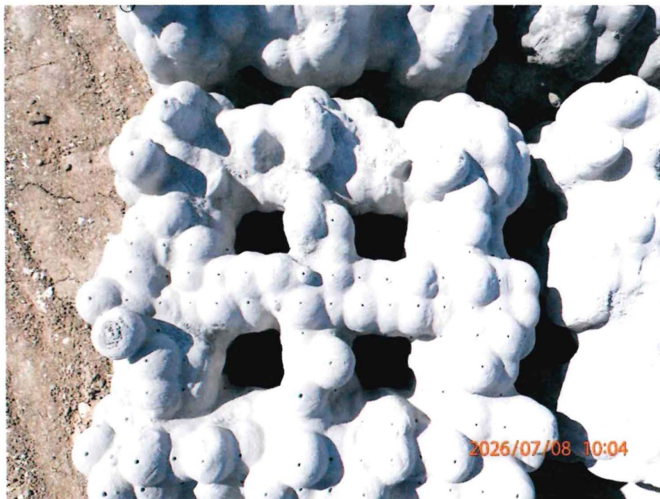
Figure 2. Top-down view of ARU showing no apparent damage.
