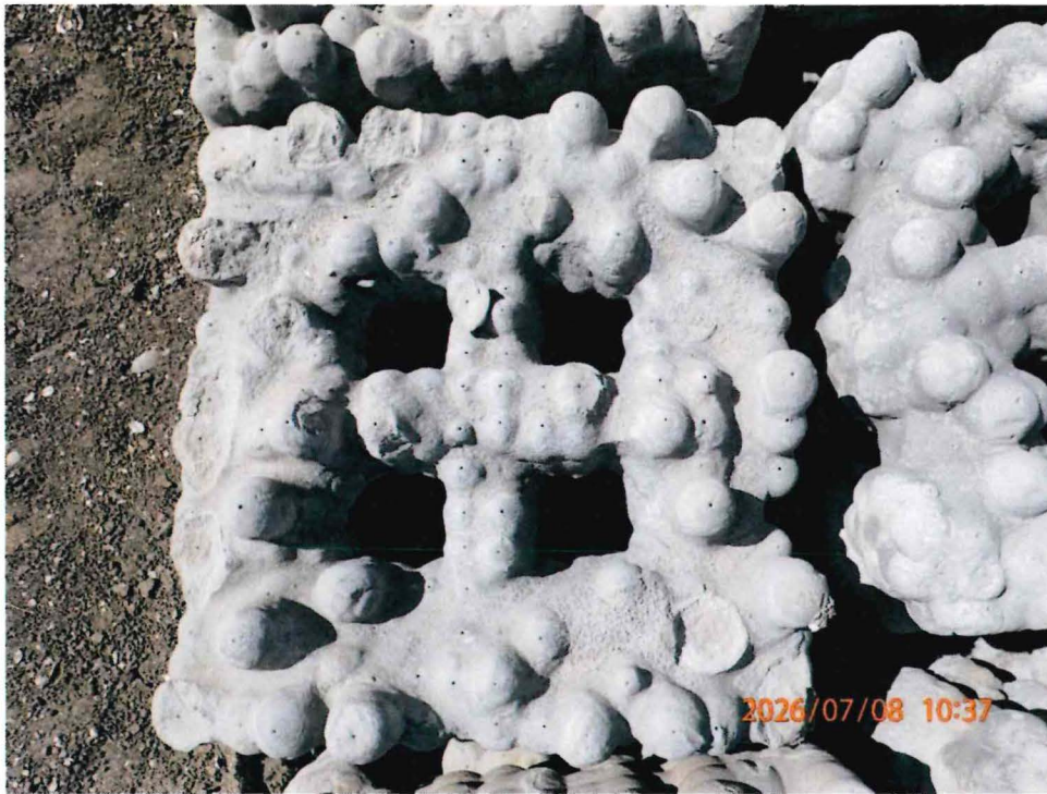
Figure 3. Top-down view of ARU showing ~41% (14/34 nodules) apparent damage.
