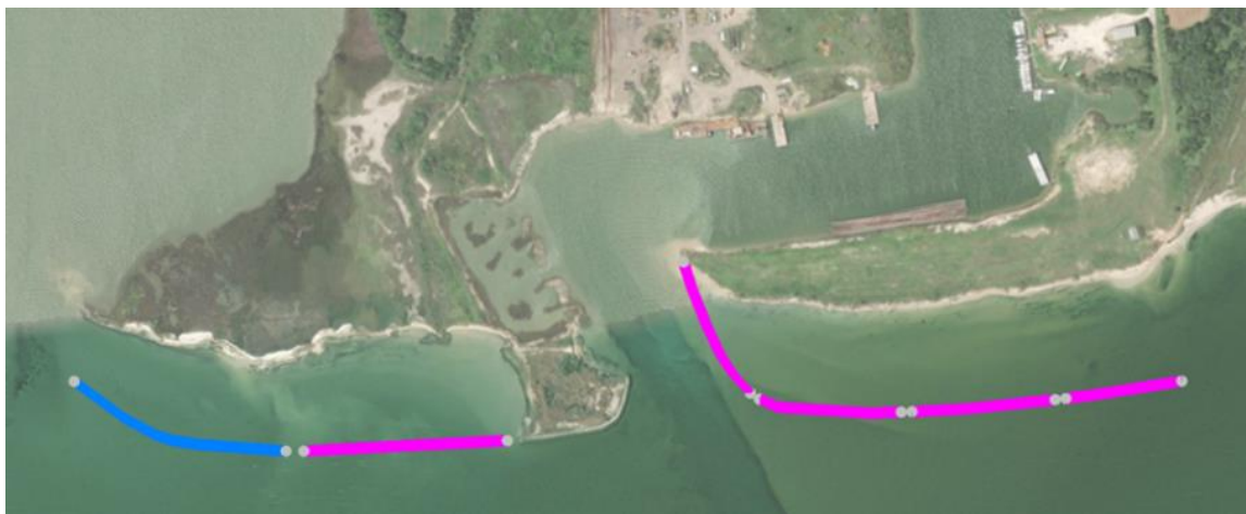
Figure 4.5: Alternative 3B breakwater configuration. Rubble mound breakwater is shown as the magenta line and artificial reef unit breakwater is shown as the blue line.
