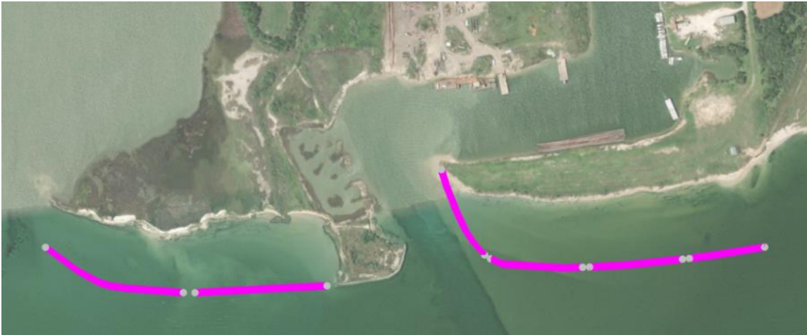
Figure 4.2: Alternative 1 breakwater configuration. Rubble mound breakwater is shown as the magenta line.
