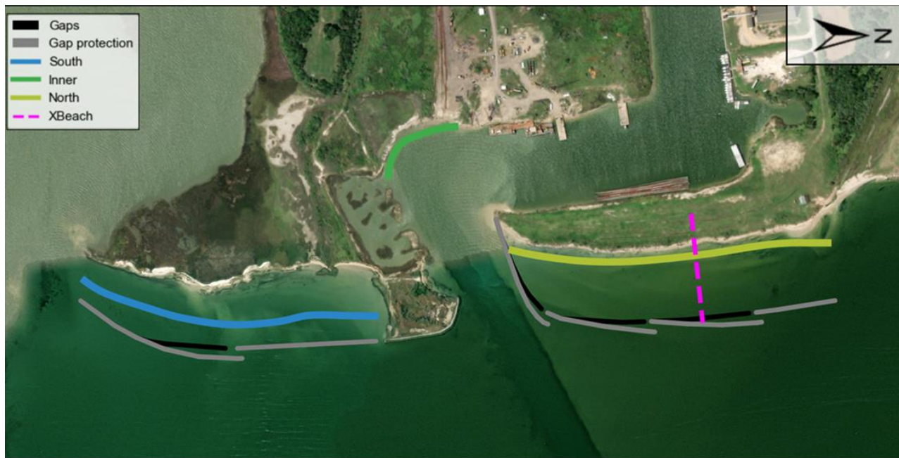
Figure 3.3: Detailed wave model features and alternative alignments. The black lines indicate the alignment for Alternatives 1, 3A, and 3B and the gray line represents Alternative 2 (see Section 5 for the alternative analysis.) The dashed pink line is the XBeach model domain (see Section 3.3 for the XBeach modeling). The remaining lines represent analysis arcs for the alternatives analysis.
