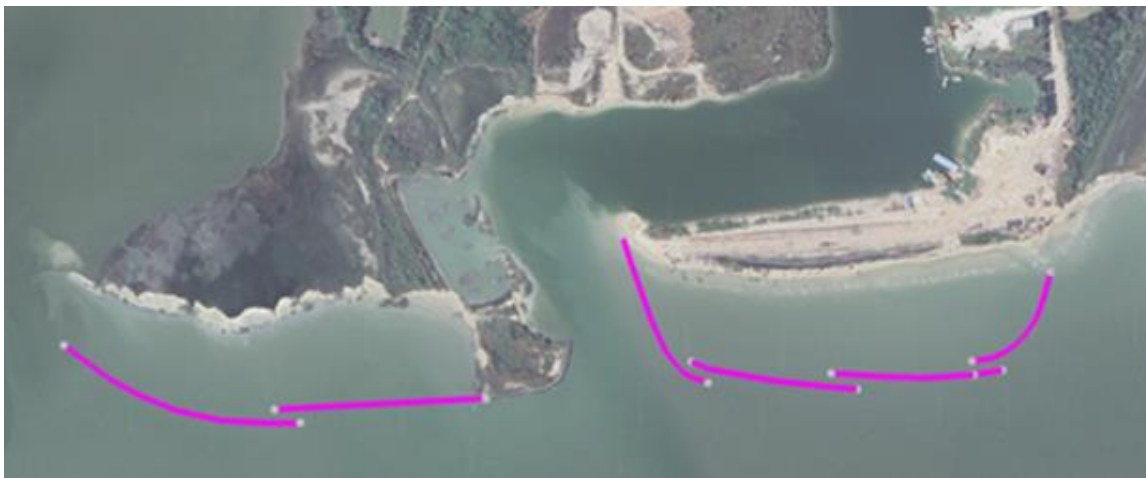
Figure 5.11: Alternative 4A breakwater configuration. Rubble mound breakwater is shown as the magenta line.
