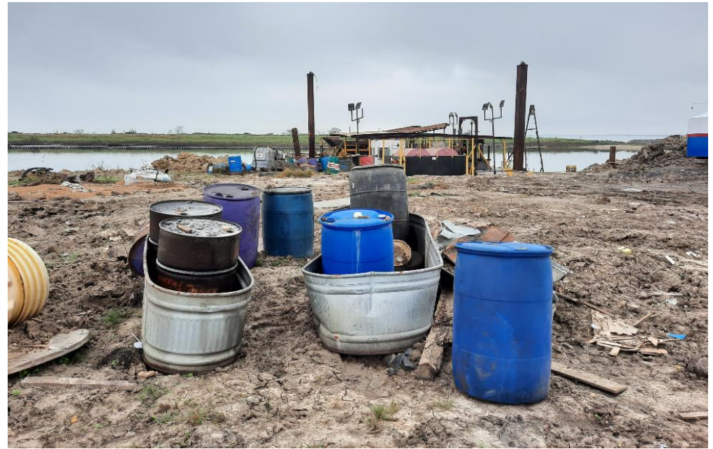
No. 6 Drum storage with secondary containment.
