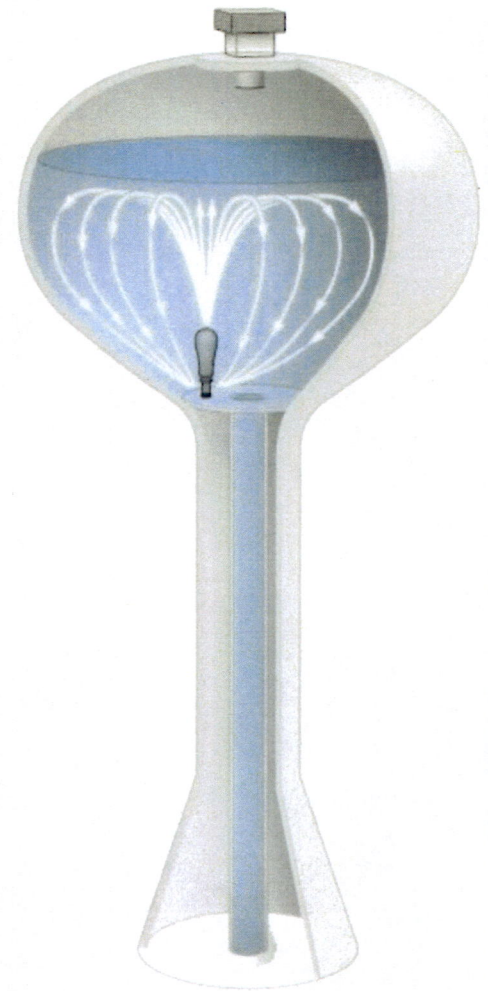
Active mixing and ventilation are the first steps in THM removal. The PAX Mixer continually introduces THM-concentrated water to the surface where THMs are volatilized and evacuated by the PAX Coaxial Powervent®.
