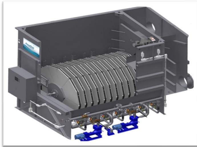
Figure 2: Aqua-Aerobic Systems AquaDisc Cloth Media Filter.
