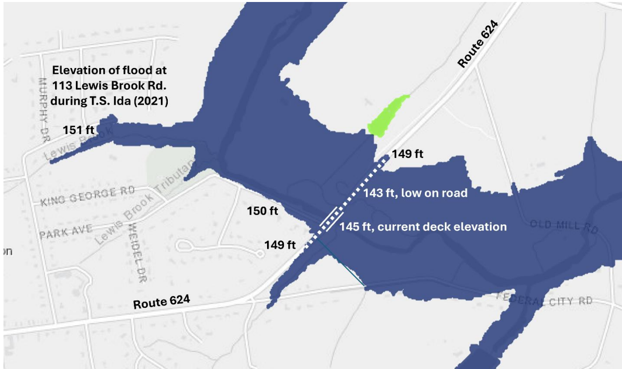
Figure 1. NJ flood elevation (2023) flood in the area of the Stony Brook bridge.
