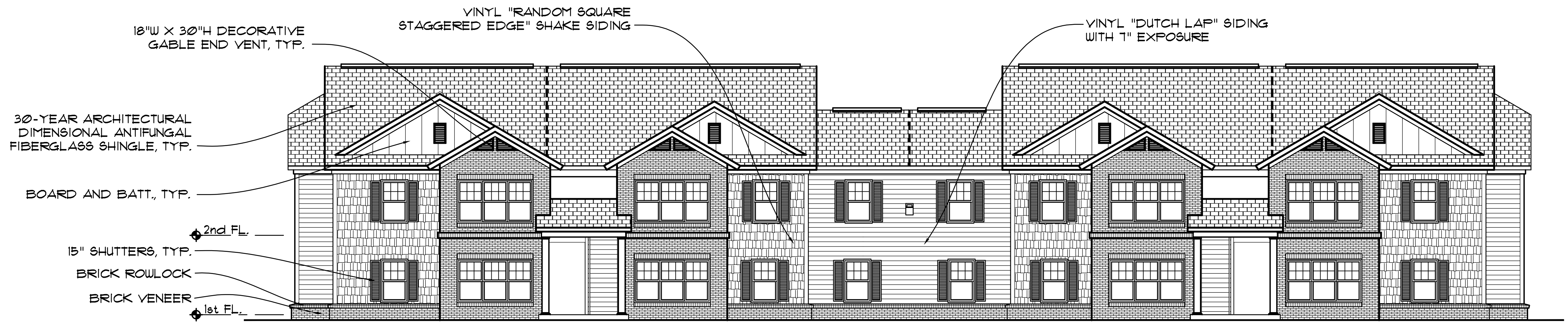
1 BUILDING 300 - FRONT ELEVATION 1/8" = 1'-0"
