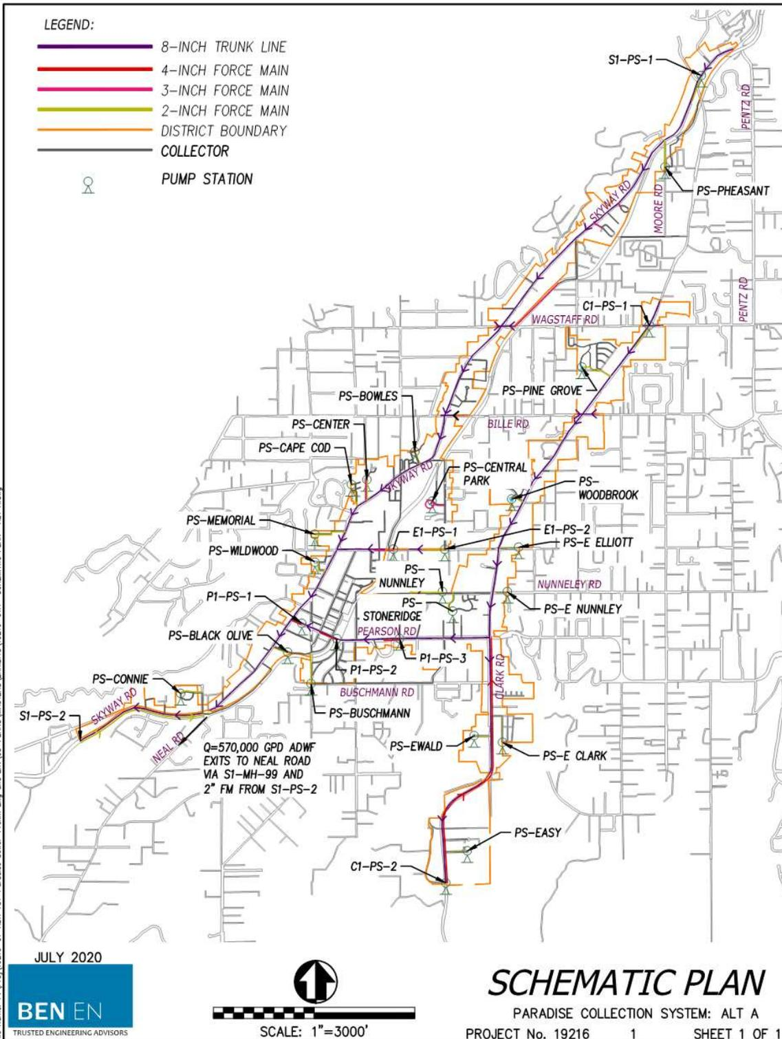
Figure 3. Schematic of Collection System – Alternative A
