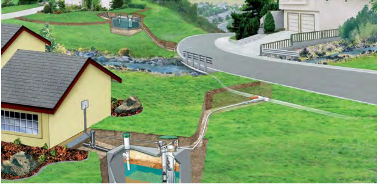
Figure 5.3 – STEP and STEG Collection Systems
