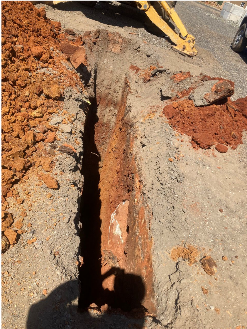
Photo No. 1 Typical test pit soil color gradation and cuttings; boulder in sidewall
