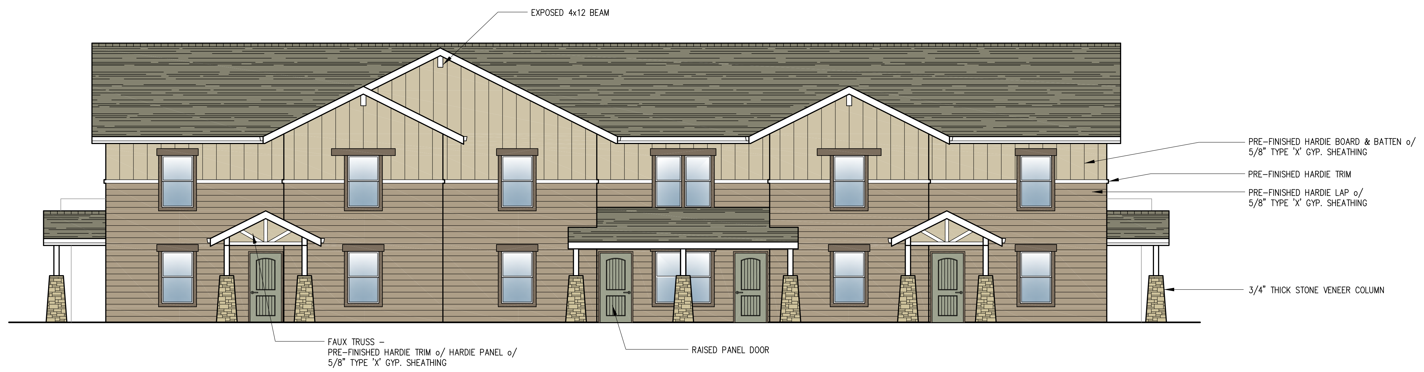
3 BUILDING D – EXTERIOR ELEVATION FRONT
