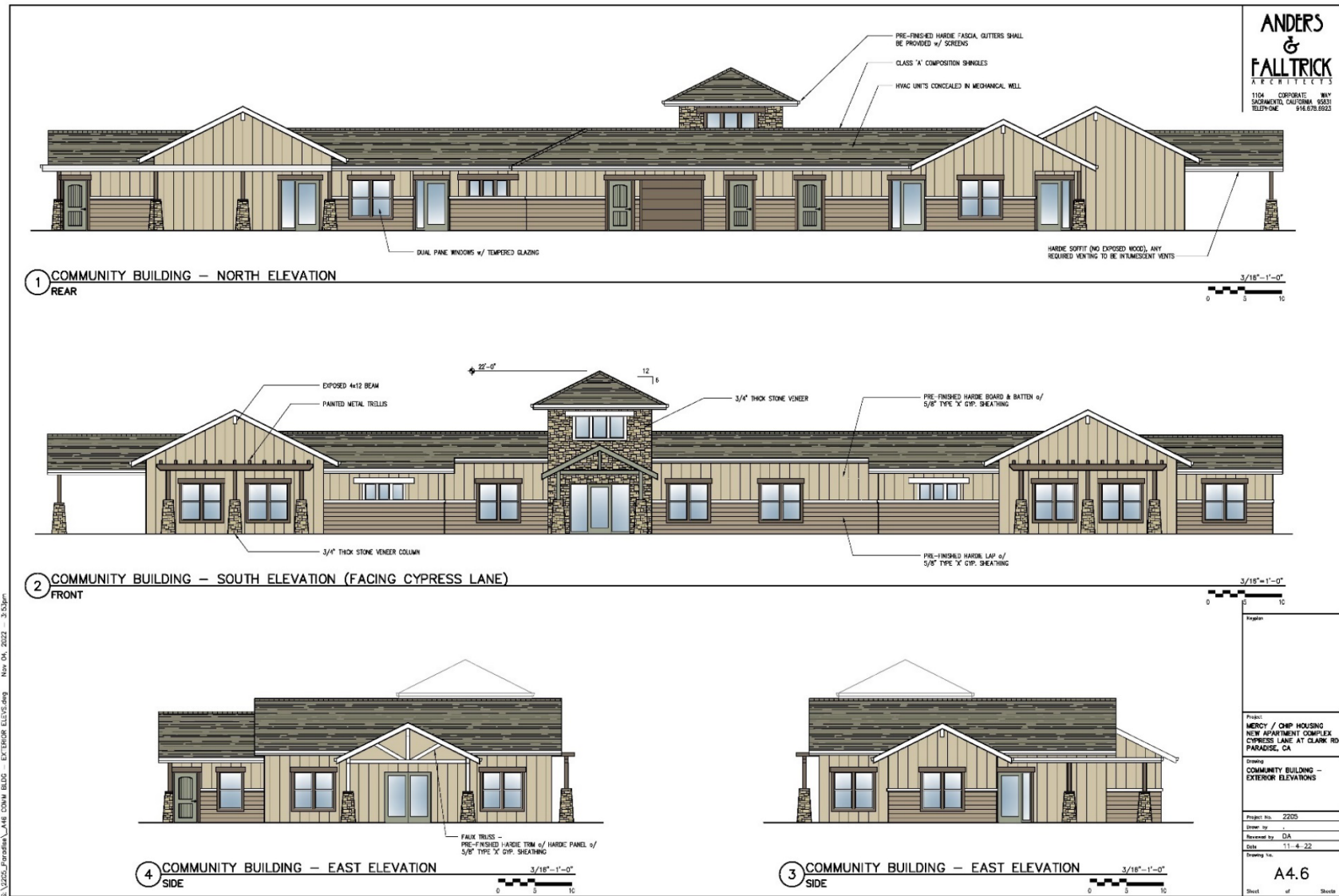
Figure 9. Community Building Elevations
