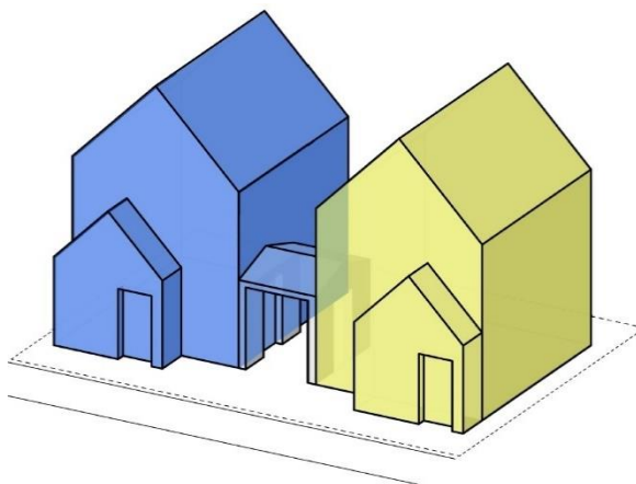
Figure 5. Duplex Attached by Breezeway
