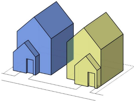
Figure 7. Detached Duplex Units Side-by-Side
