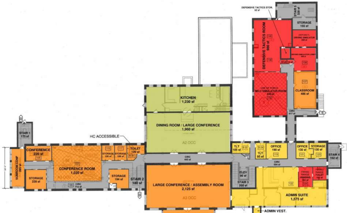
Figure 2 First Floor Existing Use Plan
