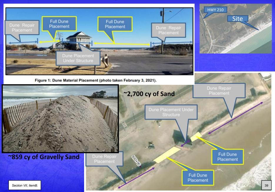
Figure 2: Plan view dune placement schematic.
