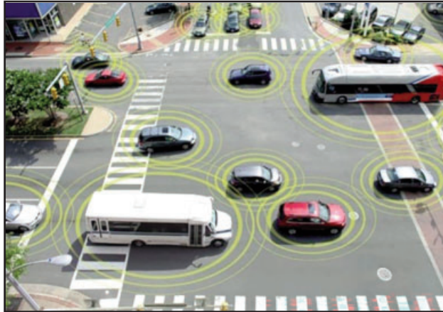
An illustration of how connected-vehicle technology shares data between vehicles and infrastructure.
