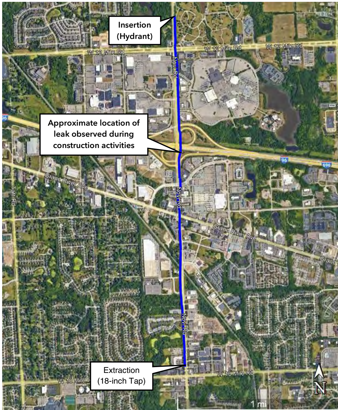
Figure 1.1: Aerial View of the 36-, 30-, and 24-inch Novi Road PCCP Water Transmission Main
