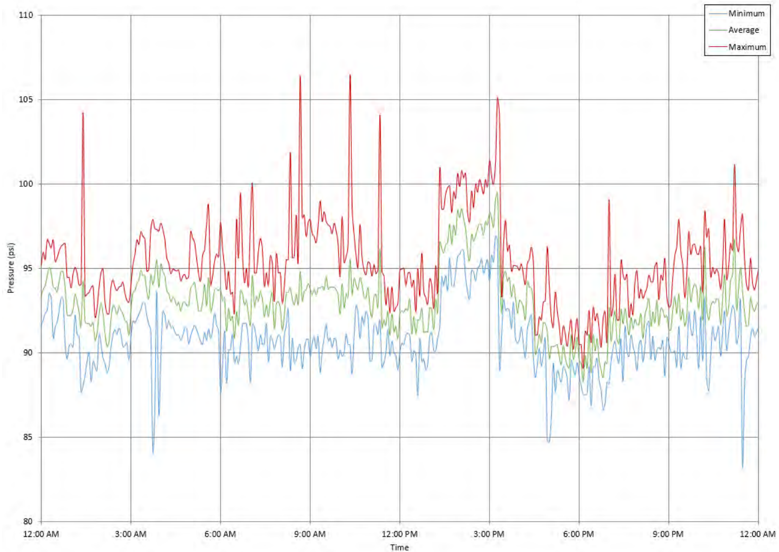
Figure 4.5: Novi Road Transmission Main (near NV-04) TPM Data - Sample Data (3/18/20).
