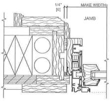
INSULATE ALL VOIDS AT WINDOW PERIMETER (BY OTHERS). SEAL UNIT TO EXTERIOR / BLIND STOP.
