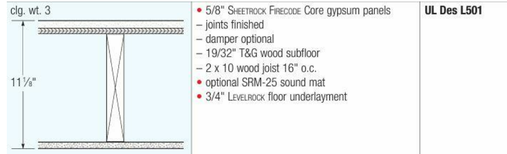
2 UL L501 - Horizontal 1HR Assembly 1 1/2" = 1'-0"
