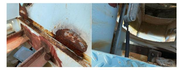
The gap between the hood structure and circular deckplate appears to be between 0 to 3". Over time, the hood structure should have some compression which results in a clearance between  $\frac{1}{2}$ " to 1". However, your clearance is much larger. Fixing this issue relates to making sure that the side rollers and the rack and track are aligned. When happens with this large opening is that excessive flow bypass the secondary mix zone.
