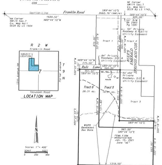
NOTE: Bearings shown are based on a Bearing of S89°44′10″E between existing monuments on the North line of the NW1/4 of Section 7, I9N, R2W, I.M. Norman, Cleveland County, Oklahoma.
