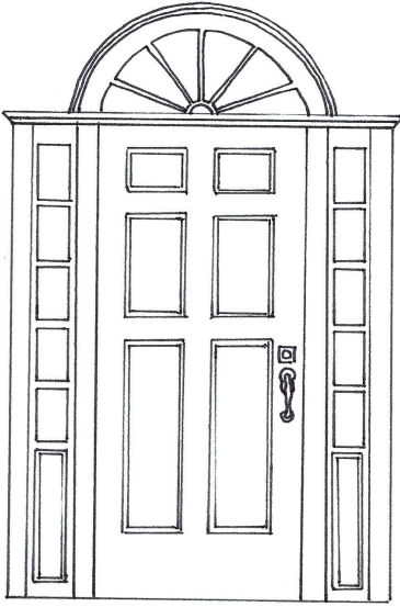
A six-panel door with sidelights and a fan light with tracery typifies Colonial Revival style.
