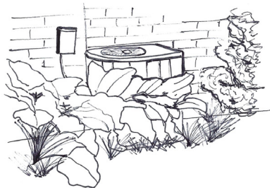
HVAC unit with planted screen
