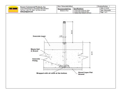
Greater degree of safety for retractable bollards because of deeper hole
