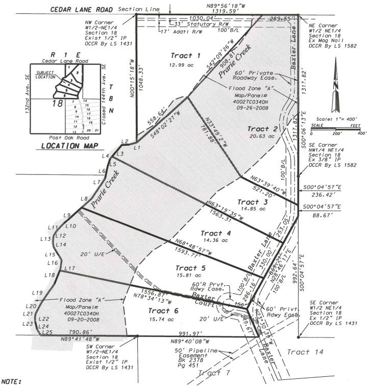
Bearings Shown are Based on an Arbitrary Bearing of N89°56′18″W Between Existing Monuments on the North line of the W/2-NE/4 of Section 18, T8N, R1E, I.M., Cleveland County, Oklahoma.
