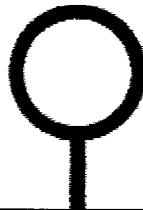
POST AND LOOP One rack element supports two bikes.
