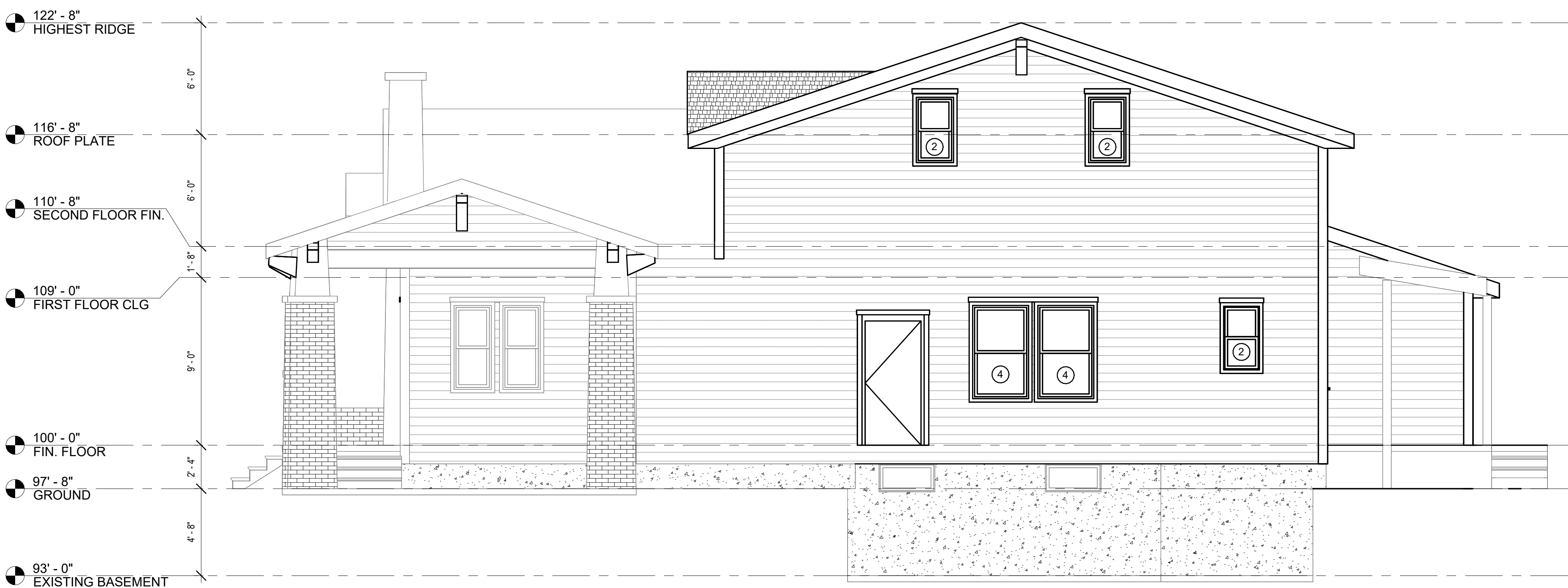
2 RIGHT EAST EXTERIOR ELEVATION 1/4" = 1'-0"
