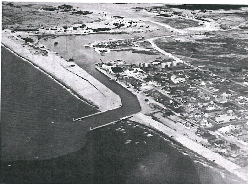
Photo 2 – Nome Harbor and Seawall – June 1955. Note narrow starved beach on the east side of the breach. Note wide beach west side of the breach as the result of littoral processes.
