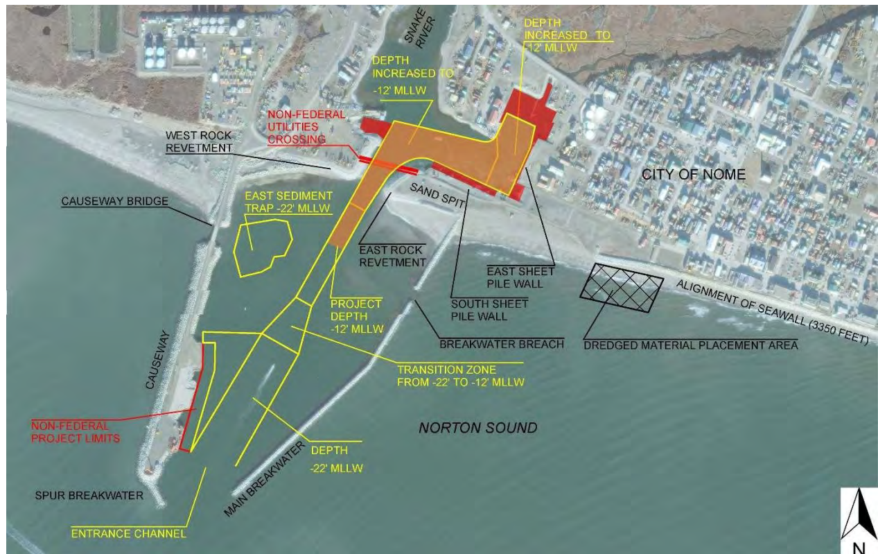
Figure 4: The Likely Recommended Plan (highlighted orange) would involve dredging in the Inner Harbor's current Federal limits, approach lane, and the Barge Ramp approach. The area in orange would have the depth increased from the current -10 ft MLLW to a new depth of -12 ft MLLW. The current Federal Operations and Maintenance area is outlined in yellow, Local Service Facilities and Non-Federal areas are in red.
